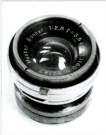
14.6 A test version of the Biogon, engraved "Muster-Sonnar" (example Sonnar) f/2.8, 35mm focal length with an internal bayonet mount.
